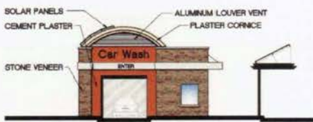
CAR WASH EAST ELEVATION
